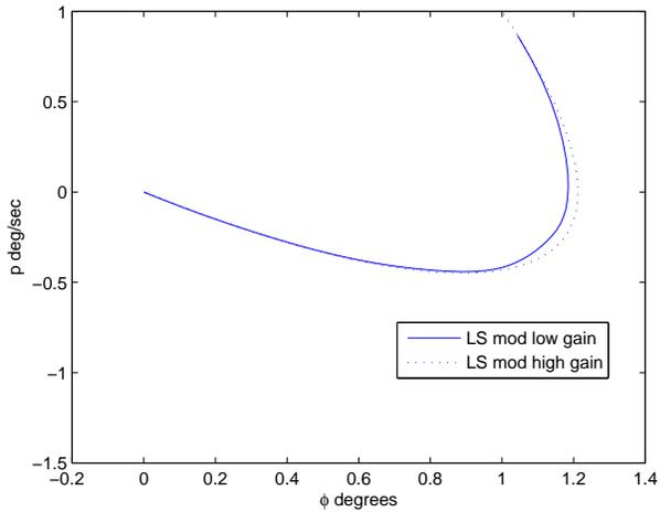
Fig. 3. Phase portrait of system states with combined direct and indirect adaptive controller
