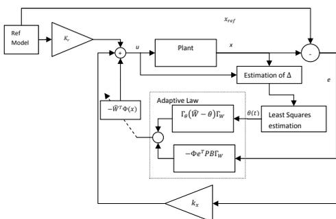
Fig. 1. Schematics of adaptive controller with recursive least squares Modification
