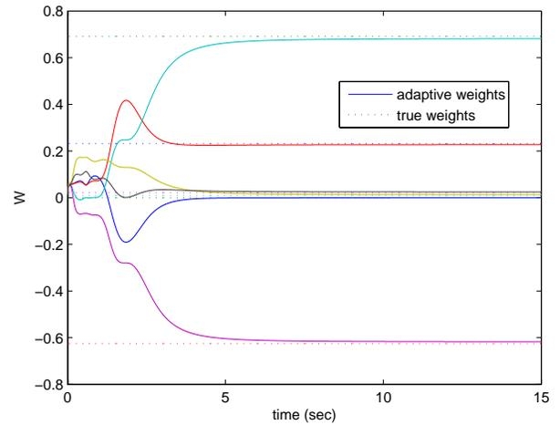
Fig. 5. Evolution of adaptive weights with combined direct and indirect adaptive controller
