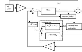
Fig. 1. Schematics of adaptive controller with least squares Modification
