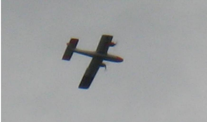
**Fig. 5 GT Twinstar in autonomous flight after jettisoning 50% of its right wing in autonomous flight to simulate severe structural damage**
