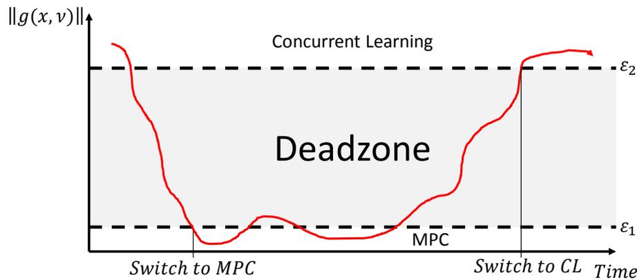
**Figure 2. Graphical interpretation of a deadzone based switching algorithm between concurrent learning and MPC.**
