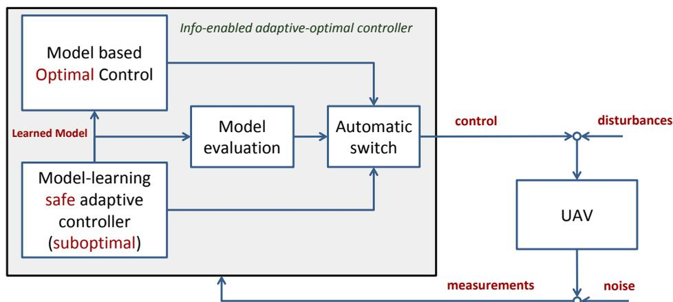
**Figure 1.** An adaptive-optimal control architecture. A learning-focused adaptive controller guarantees stability while learning uncertain system parameters. Once sufficient confidence has been gauged online in the estimated parameters, the architecture switches to using an online model-based controller, such as MPC. The resulting switched adaptive-optimal controller is guaranteed to be stable without being conservative about initial parameter errors.
