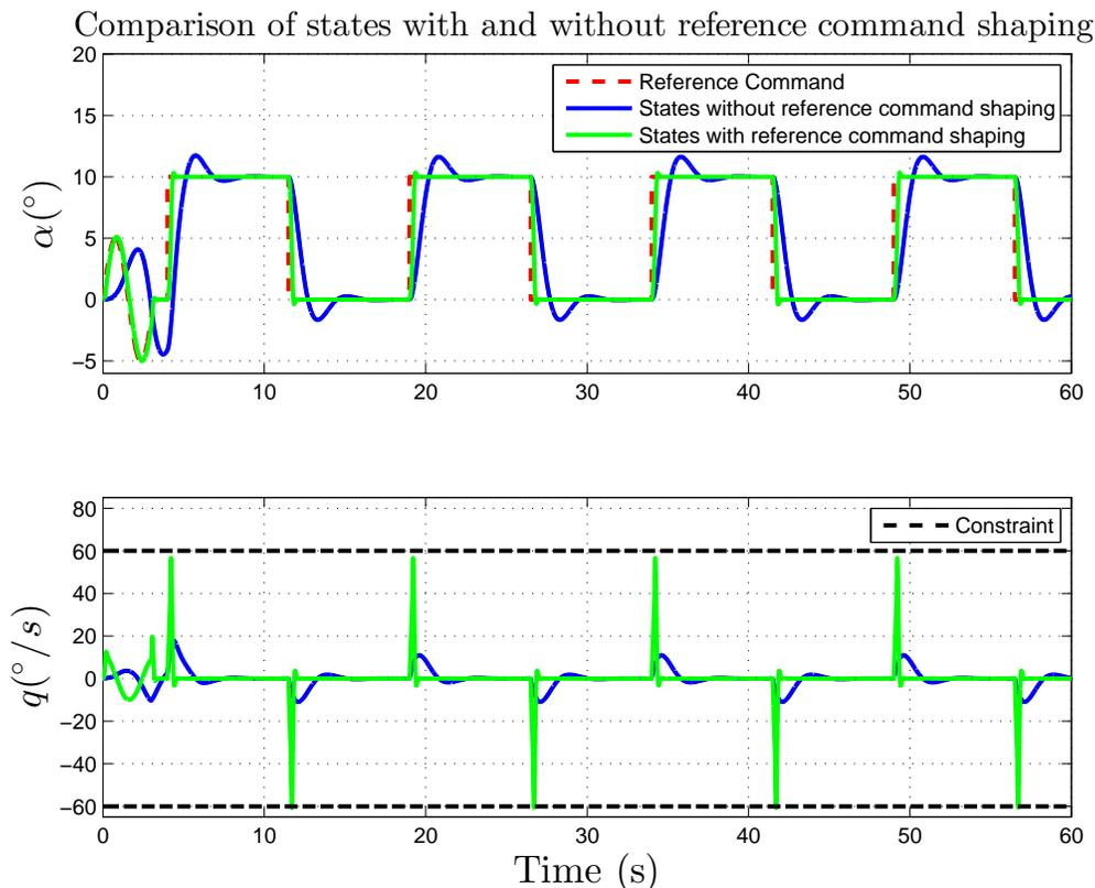
**Figure 2. Comparison of states with and without reference command shaping. It can be seen that the performance increases drastically if the reference command is shaped such that the linear reference model is controlled optimally. Simultaneously the constraint on the pitch rate is abided.**
