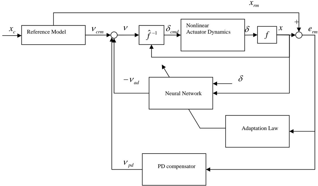
Figure 1. Neural Network Adaptive Control using Approximate Model Inversion
