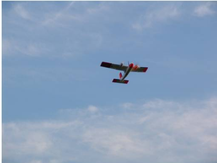
Figure 3. The Georgia Tech Twinstar UAS in autonomous flight with 25% of the left wing missing.
