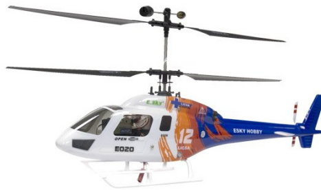
Figure 3. The Esky E020 “Big Lama” coaxial helicopter. Note: the tail rotor on this aircraft is neither functional nor required for flight.
