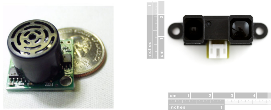
Figure 5. Primary range sensors are the MaxBotix® LV-MaxSonar® (on the left), and the SHARP GP2Y0A02YK0F infrared range sensor (on the right). Photos courtesy SparkFun Electronics: www.sparkfun.com .
