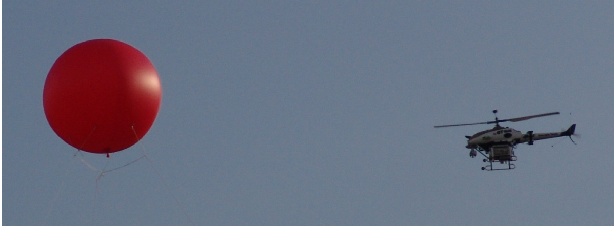
Figure 1. The GT Max UAV performing vision-based target tracking and obstacle avoidance using a weather balloon.
